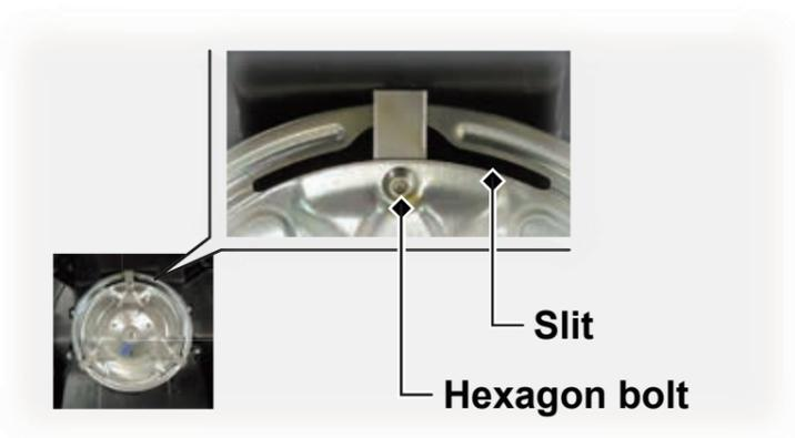
Blade Replacement - Disk with hexagon bolts by using the blade holder tool\*
